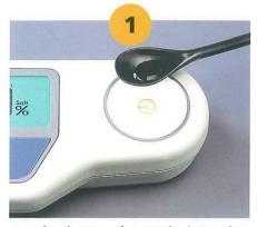
Apply drops of sample into the sensor section until it fills above the indication line.
