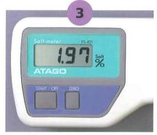
After arrow flashes three times, the display indicates the salinity of the measured sample in percentage.
