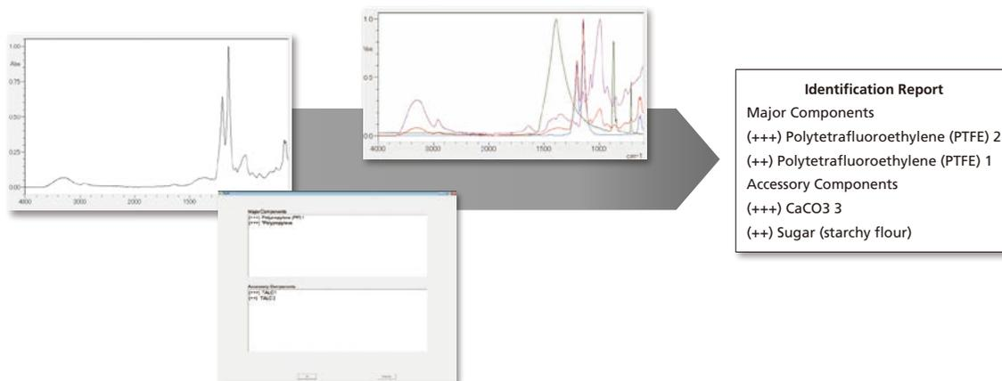
Shown here is an analysis of a contaminant attached to a tablet surface using the Contaminant Analysis Program. The results showed Polytetrafluoroethylene (PTFE) was the major component, and sugar and calcium carbonate were the accessory components. Since the two accessory components are often used as tablet components, it is estimated that the components were scraped up at the same time when scraping the contaminant.
