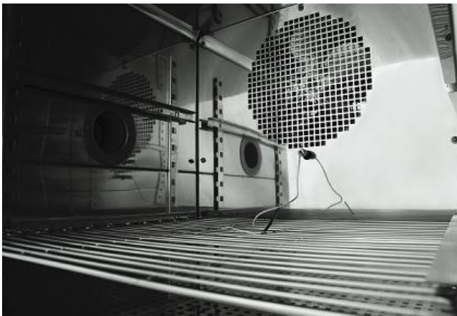
From left to right: interior of FitoClima 300 and 1.500. Visible at the images: highly resistant AISI 304 stainless steel with height adjustable shelves, port-hole and PT100 class A temperature sensor. Fans and perforated trays and interior base allow for uniform circulation and distribution of temperature and humidity inside the chamber.
