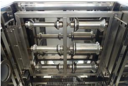
Cables/Wires winding accessory for 'Cold bend' testing
