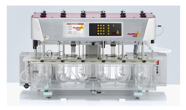
The PTWS D620 is a "Dual Drive" 6 + 6 position, single drive tablet dissolution testing instrument for solid dosage forms as described in USP chapter <711/724> and EP section<2.9.3/4> as well as the DAB/BP and Japanese Pharmacopeia section <15>. The instrument features two additional vessels (approx. 250ml) for media refilling and reference standard media. PTWS D620 features independent stirrer speed control for the front and back row of stirrers.
