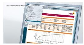
For an online automated system it is possible to use a UV/VIS spectrophotometer with a multiple-cell-changer. The spectrophotometer and pump of such a system is controlled by the powerful WinDiss ARGUS dissolution software. WinDiss ARGUS features drivers for most commonly available UV/VIS spectrometer types, like Agilent 8453 Diode Array, or conventional UV/VIS
