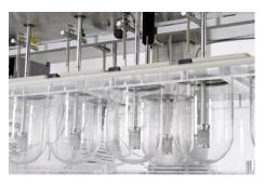
The motorized EPE-1220 sampling system lowers the sampling probes into the media and after sampling raises them back out again. 8 different sampling positions can be programmed. The ITM-1220 individual media temperature monitoring system is attached to the EPE-1220 and will read and report the vessel media temperatures while sampling.
