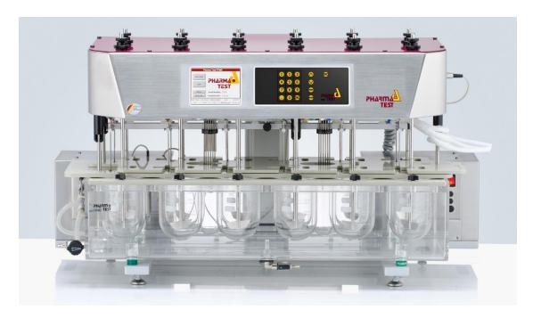
The PTWS 1220 is a 6 + 6 position, single drive tablet dissolution testing instrument for solid dosage forms as described in USP chapter <711/724> and EP section<2.9.3/4> as well as the DAB/BP and Japanese Pharmacopeia section <15>. The instrument features two additional vessels (approx. 250ml) for media refilling and reference standard media. The PTWS 1220 is the ideal choice for Biowaiver studies and dissolution method development.
