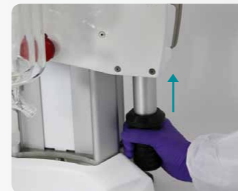
No-tools vessel height adjustment
