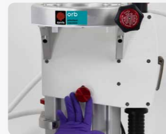
No-tools vessel height adjustment
