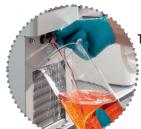
**Tidy.** The special drain tap for easy draining of bath fluids without tools.
