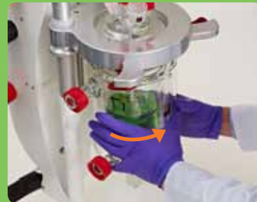
Easy to raise/lower stirrer motor and auto aligning stirrer
