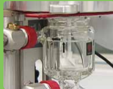
Quick oil pipe connection and oil pipe tidy
