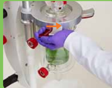
Easy to raise/lower stirrer motor and auto aligning stirrer
