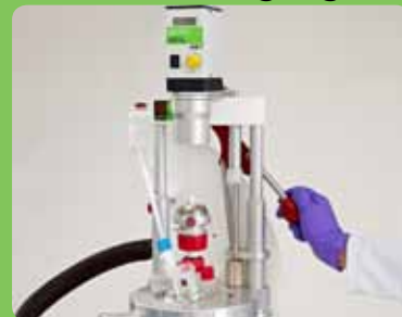
Easy to raise/lower stirrer motor and auto aligning stirrer
