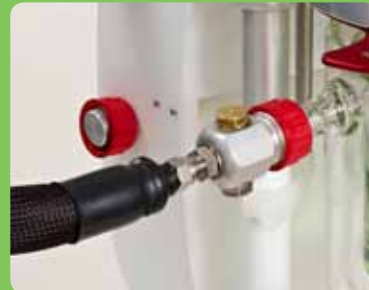
Quick vessel clamp and release
