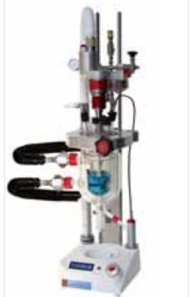
Atlas Potassium Pressure Control reactions up to 3 bar and 200°C with volumes up to 3L in a glass jacketed reactor.
