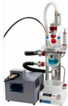
Atlas FTIR Analysis Monitor reactions in real time with an integrated mid-IR spectrometer.
