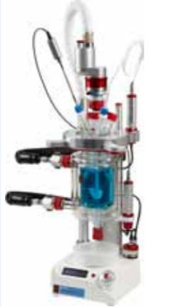
Atlas Turbidity Display and log turbidity by connecting the Atlas Turbidity Probe to the base.
