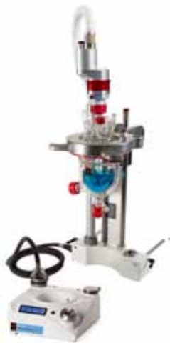
Atlas Remote Mount Locate vessels up to 5L away from the Atlas Base.
