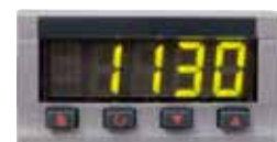
Over-temperature limit controller
