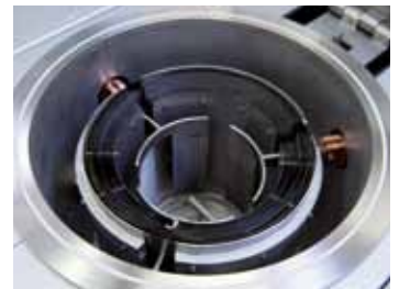
Cylindrical retort with tungsten heating
