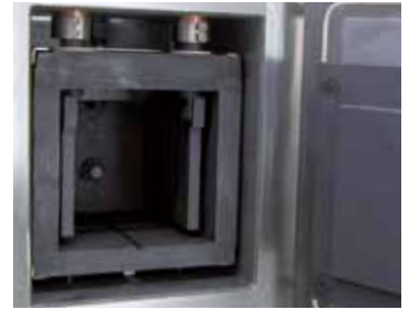
Graphite heating chamber
