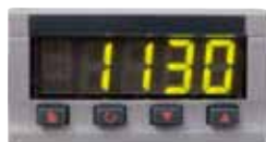
Over-temperature limit controller
