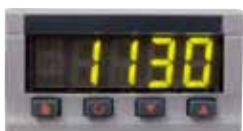
Over-temperature limit controller
