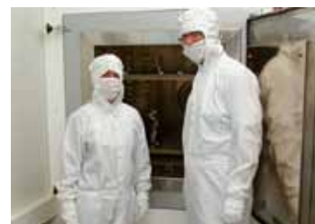
Industrial oven N 250/65 HAC with particle-free oven chamber. For charging, furnace door is located in cleanroom, class 100, furnace chamber in greyroom behind.
