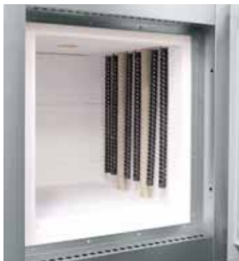
Vertically mounted SiC rods
