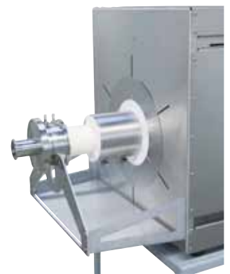
Gas-tight design with water-cooled flanges
