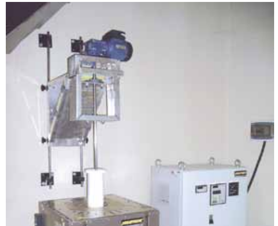
RHTV 120/300/15 integrated in a tensile strength testing machine
