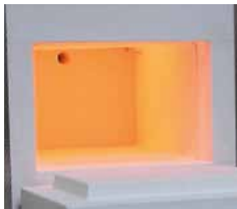
Muffle heated from four sides
