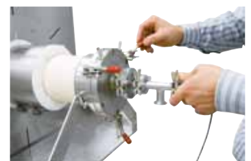
Water-cooled end flange with quick connectors as additional equipment
