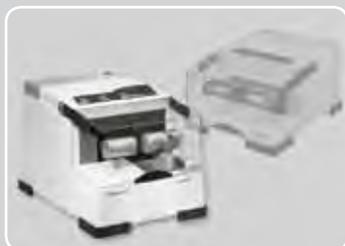
Fine size reduction with impact and friction can also be carried out with RETSCH Mixer Mills. They are used for **small sample volumes and cryogenic grinding**.
