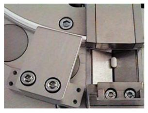
The unique feature of the WHT 3ME is the movable FLAP device. It positions precisely within the Length/Hardness test station.
