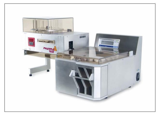
Test WEIGHT, THICKNESS, DIAMETER (or LENGTH), and HARDNESS of regular tablets, odd shaped tablets (caplets, oblongs etc.) and other solid samples fully automatically.
