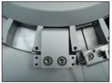
For sample transportation a carousel is used which has 20 segments, each of which takes a tablet. Each segment is equipped with a PTFE scraper to clean the hardness testing jaws from cohesive products and to clean the track of residual particles.
