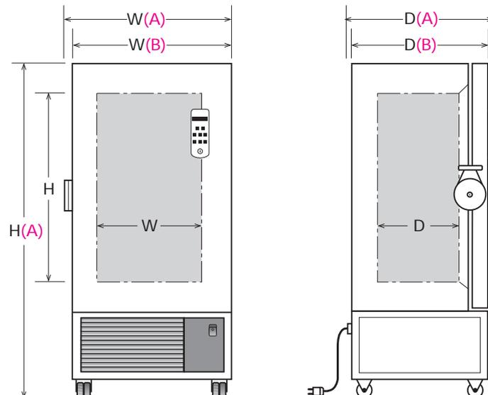
Sometimes, narrow doors demand smaller unit widths and/or depths when the Freezers are transported to the place of use. The product table (page 16) shows both dimensions (A and B), illustrated on this page.
