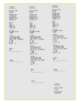
The PT-TD200 is equipped as standard with an RS232 COM and a USB/s port which allows the connection of a PT-DL1 Data Logger and the update of the system in case this will become necessary any time. Connecting the serial PT-DL1 printer enables the print-out of a report of test results including the detailed description of the used testing method, operator (if activated) and the results including volume and weight information.
