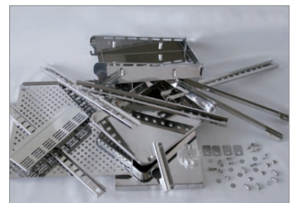
Dismantled inner parts of a conventional CO 2 incubator demonstrates the huge amounts of contaminateable surface.
