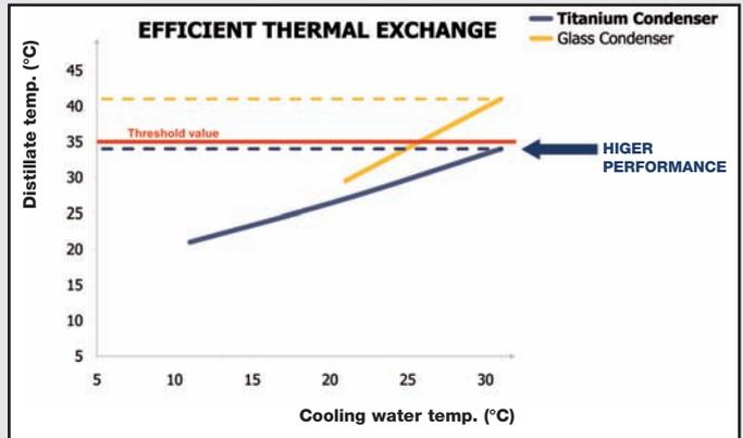
\* Tap water flow rate 1 l/min
