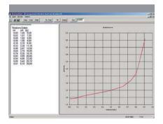
With the TitroLine Chart software (option), the titration curve can be displayed on the monitor of a connected PC and the titration data can be processed.
