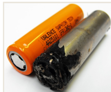
AA Batteries after a test in a ‘Standard’ BTC .
