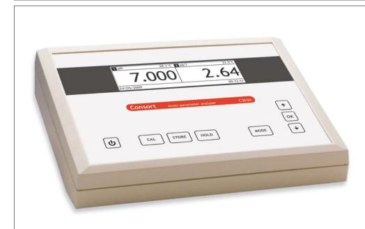
pH: -2...+16 pH mV: ±2000 mV 0.01 ng/l...100 g/l lon: Conductivity: 0...2000 mS/cm Resistivity: 0...200 MΩ.cm 0.0...70.0 Salinity: TDS: 0...100 g/l 0...60 mg/l Dissolved oxygen:
