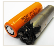
AA Batteries after a test in a 'Standard' BTC.
