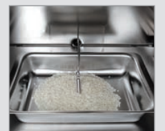
Specimen temperature display with PT 100 sensor (ED | FD | FED | FP | M | VD | VDL)
