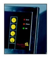
Red - yellow - and green "traffic" lights inform the user from anywhere in the laboratory of the instrument's status. Yellow will light up if any specification is slightly outside the limits but with no major problem for the correct performance of the dissolution run. The red light comes on as soon as any critical fault has been found which would surely question the validity results of test results, such as incorrect stirrer position etc.
