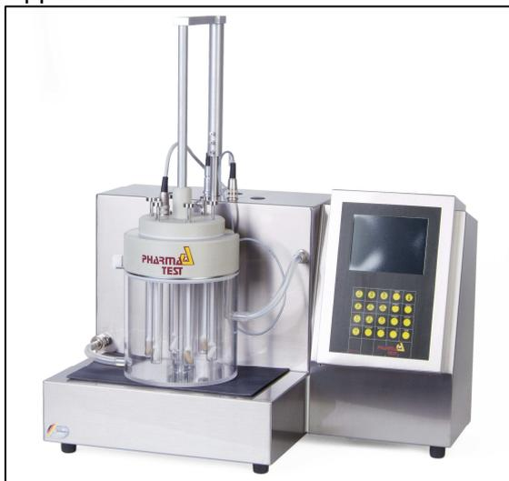
The Apparatus is placed into a single position Plexiglas water bath. So it possible to use the SPT-6 in the Tablet Disintegration Apparatus PTZAUTO 1 - 4 and 1EZ - 4EZ as well as in the PTZS. Using the SPT-6 within a PTZ AUTO EZ system the softening time can be detected and reported automatically.
