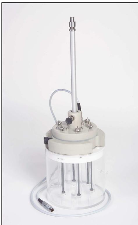
The **SPT-6** Suppository Penetration Test Assembly is used to determine the softening time of 6 samples at the same time and has to be connected to a Pharma Test Tablet Disintegration Instrument PTZAUTO or a PTZS. The SPT-6 Assembly can also be immersed into a suitable water bath. The SPT-6 is made in strict compliance with the monograph of the EP <2.9.22> Apparatus <A>.
