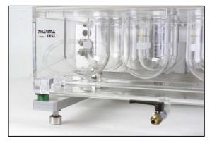
dosage manufacturing of solid forms. transdermals, ointments and creams. Nearly suppositories etc. all international pharmacopoeias describe a dissolution test instrument, in which at least 6 samples should be tested. The test vessel design, stirring speed range, temperature range and accuracy, stirrer design and relevant tolerances are clearly specified.
