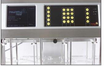
running well = green light - slight problem = yellow or out of specification = red. All this is automatically logged; the log file can be printed any time using the built-in thermo printer.
