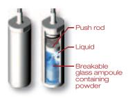
• Ampoule vessel to study powder wetting or hydration.
