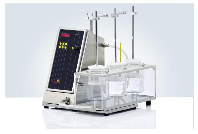
The **DIST3** is a three-basket manual tablet disintegration testing instrument, manufactured according to the recent **USP** <701/2040>, **EP** <2.9.1/2.9.1.2>, JP and other pharmacopoeias.
