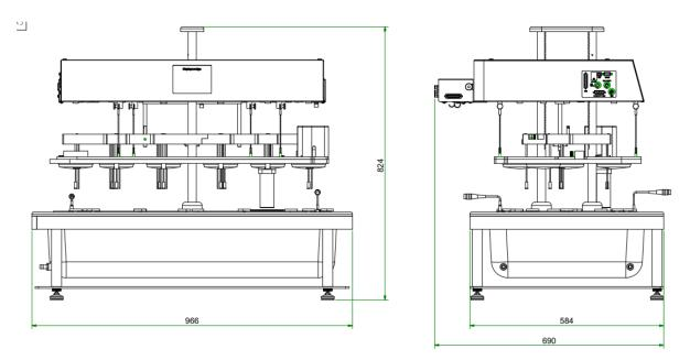
With less than 100cm of total width for the main instrument, PTWS 1420 features a sturdy design and yet makes optimal use of the limited space available in a typical laboratory.
