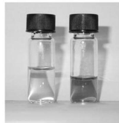
Figure 5. Collection of the two phases after phase separation in continuous flow: aqueous phase containing EDTA, copper, and NMP (left vial), and the organic phase containing triazole (right vial).
