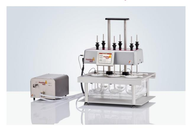
The PTWS 120D is a 6 position, single drive compact tablet dissolution testing instrument for solid dosage forms as described in USP chapter <711/724> and EP section <2.9.3/4> as well as the BP, DAB and Japanese Pharmacopeia section <15>.Its design for manual operation and ease of use.
