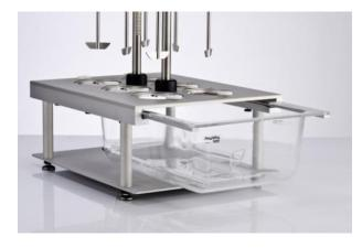
The vacuum molded water bath can easily be removed from the support frame for cleaning purposes. The bath cover can also be easily unscrewed for cleaning. The water bath contains a water diffuser for faster heating and to ensure that heated water is evenly distributed throughout the whole bath. Optionally a double walled vacuum molded water bath is available which reduces the heat transfer to the outer environment to save internal heating and external cooling energy
