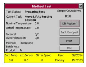
parameters can be tool speed, target bath temperature, sampling time points and so on. The test method memory capacity is almost limitless. As soon as the test is started, a screen saver can be
