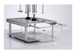
The vacuum moulded water bath can easily be removed from the support frame for cleaning purposes. The bath cover can also be easily unscrewed for cleaning. The water bath contains a **water diffuser** for faster heating and to ensure that heated water is evenly distributed throughout the whole bath. Optionally a **double walled** vacuum moulded water bath is available which reduces the heat transfer to the outer environment to save internal heating and external cooling energy
