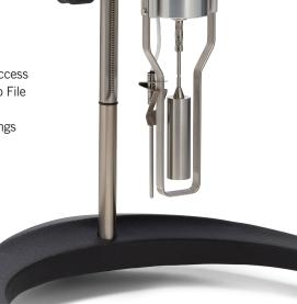
Analyze characteristics such as yield stress, flow curves (mixing, pumping, spraying), leveling and recovery
