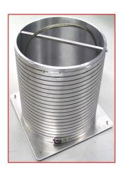
The Joule effect calibration system allows for the dissipation of a predefined power level between of 30 mW to 13 W. Calibration by Joule effect uses an electrical cell consisting of a resistive element wound around a metal cylinder. A constant level of power is dissipated in the sensitive area of the instrument. The calculation of the relation between the calorimetric signal ( $\mu$ V) and the power (mW) gives the calibration coefficient ( $\mu$ V /mW) at an isothermal temperature.
