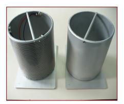
The Joule effect calibration system allows for the dissipation of a predefined power level between of 30 mW to 3 W. Calibration by Joule effect uses an electrical cell consisting of a resistive element all around a metal cylinder. A constant level of power is dissipated in the sensitive area of the instrument. The calculation of the relation between the calorimetric signal ( $\mu$ V) and the power (mW) gives the calibration coefficient ( $\mu$ V /mW) at an isothermal temperature.
