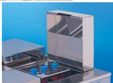
Double-walled lid with inner camber have insulating capacity and prevent dripping back of condensate into the vessels
