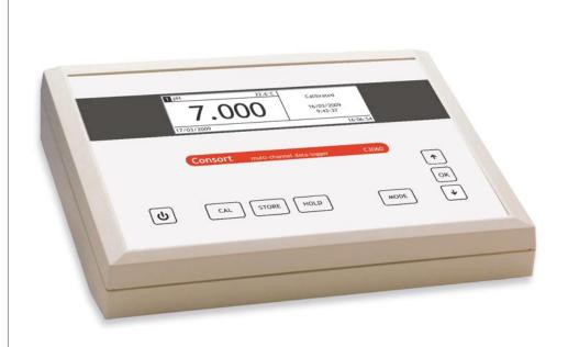
pH: -2...+16 pH mV: ±2000 mV 0.01 ng/l...100 g/l lon. Conductivity: 0...2000 mS/cm Resistivity: 0...200 MΩ.cm 0.0...70.0 Salinity: TDS: 0...100 g/l -5...+105°C Temperature:
