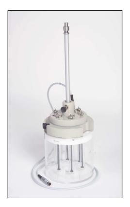
The **SPT-6** Suppository Penetration Test Assembly is used to determine the softening time of 6 samples at the same time and has to be connected to a Pharma Test Tablet Disintegration Instrument PTZAUTO or a PTZS. The SPT-6 Assembly can also be immersed into a suitable water bath. The SPT-6 is made in strict compliance with the monograph of the EP <2.9.22> Apparatus <A>.
