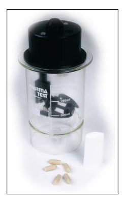
The **PTSW-0** Suppository Dissolution Test Cell (Rotating Dialysis Cell) is placed into a normal USP type dissolution vessel placed into a dissolution bath to test the rate of dissolved active of suppositories and lypophilic carriers.
