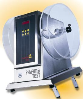
We offer to the user a series of instruments to meet his requirements. Each of the instruments can be optionally equipped with an Abrasion Drum having a diameter of 20 cm and inside 12 lamellas. The standard Friability Drum
